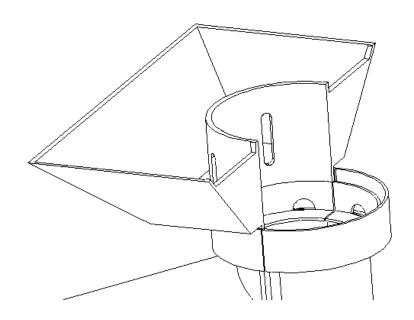
Install side two into Collar Position vertically and slide into place
