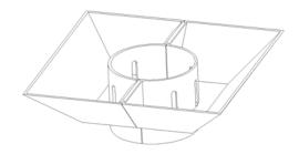
The Top Tray is installed in such a way that no seals are required to direct the fluid into the Flow Tee
